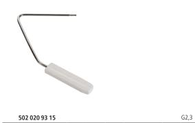
With the help of a knee lifter, the presser foot is lifted and the feed dog is lowered at the same time. This also increases the gap between stitch plate and presser foot, and leaves both hands free to guide your project.
