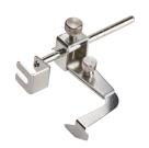
The adjustable seam guide is attached around the presser foot shaft and can be used with different presser feet. Using the two adjustment screws, the guide can be moved along the ruler line up to 1 1/2' to the right of the needle to guide sewing along an edge or a previous row of stitches.
