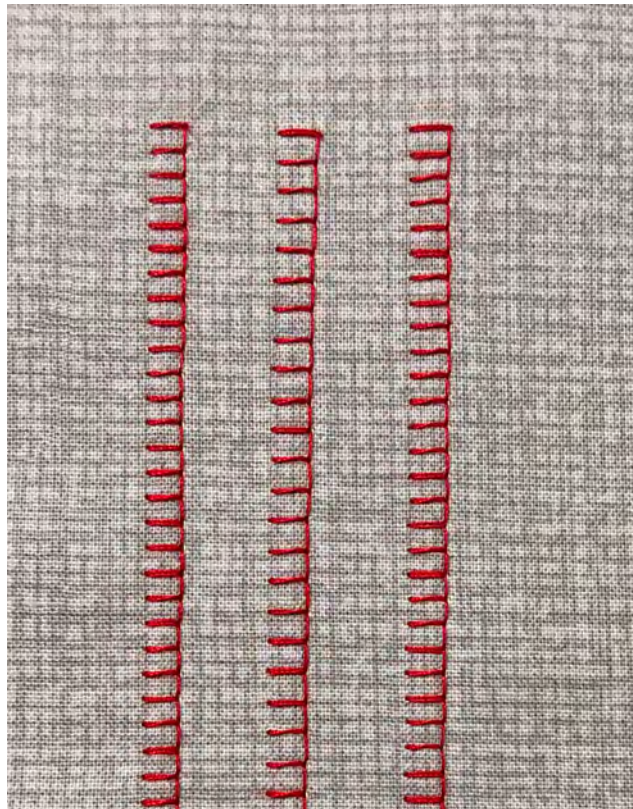
Row 1 Programmed settings Row 2 4 mm width 3 mm length Row 3 4 mm width Default length
